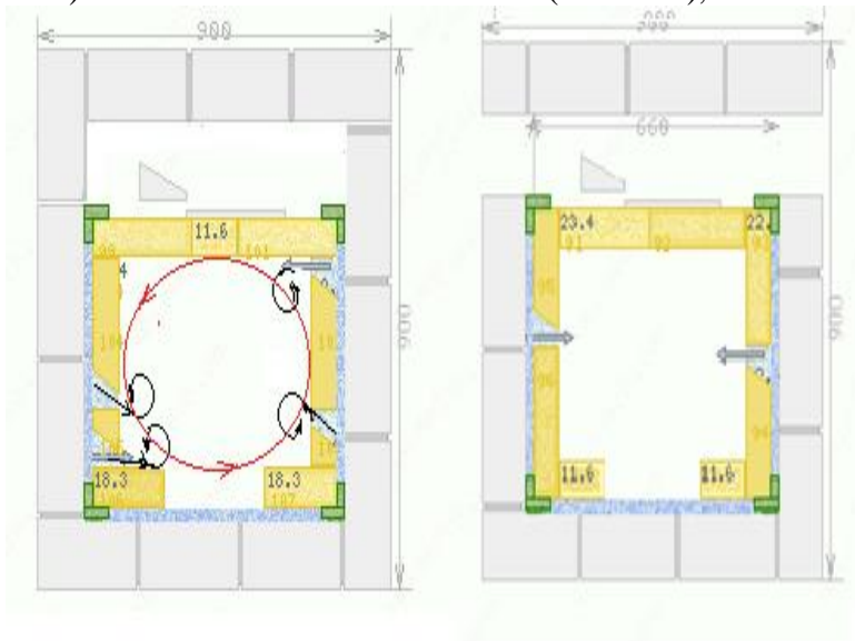
Fig. 9. VM in a house-hold furnace –the section in the area of furnace door, view from the top
