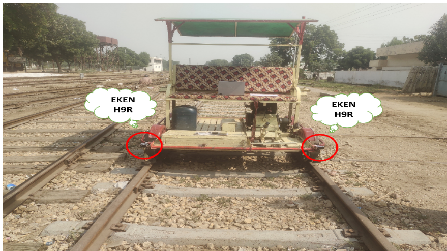
Figure 6: EKEN H9R Interfacing with Motorized Manual Track Recording Vehicle (TRV).
