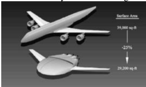
Fig.6: Effect of engine installation on surface area [1]
