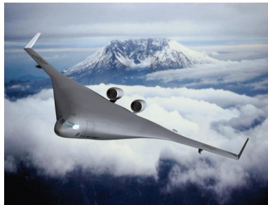
Fig.3: A Blended Wing Body Aircraft [2]
